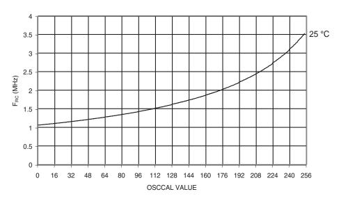
Figure 198. Calibrated 4 MHz RC Oscillator Frequency vs. Temperature
