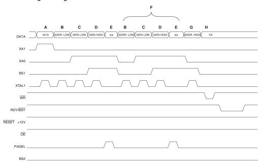
Figure 137. Programming the Flash Waveforms
