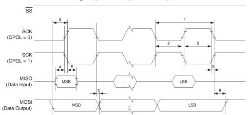
Figure 154. SPI Interface Timing Requirements (Master Mode)
