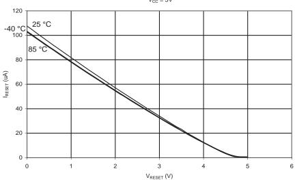
Figure 212. Reset Pull-up Resistor Current vs. Reset Pin Voltage ( $V_{CC} = 2.7V$
