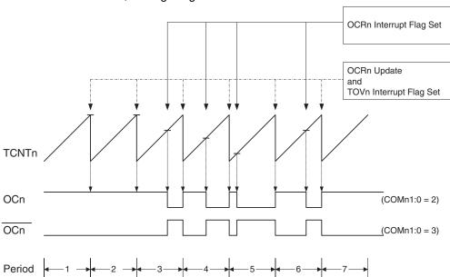
Figure 66. Fast PWM Mode, Timing Diagram
