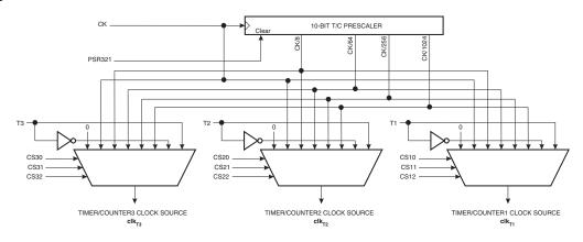
Note: The synchronization logic on the input pins (T3/T2/T1) is shown in Figure 59.
