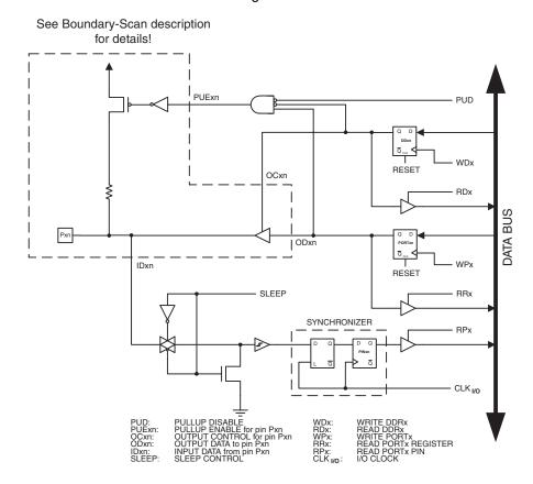
Figure 125. General Port Pin Schematic diagram
