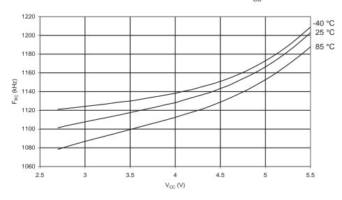
Figure 192. Calibrated 1 MHz RC Oscillator Frequency vs. Temperature
