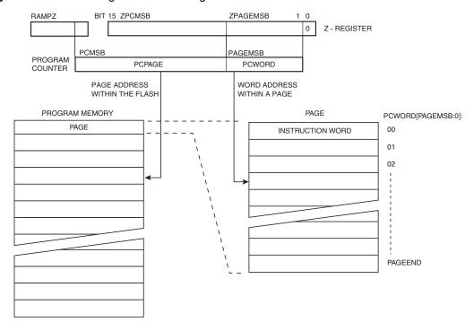
Figure 134. Addressing the Flash During SPM<sup>(1)</sup>
