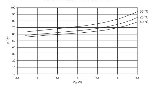
Figure 208. Programming Current vs. V<sub>CC</sub>
