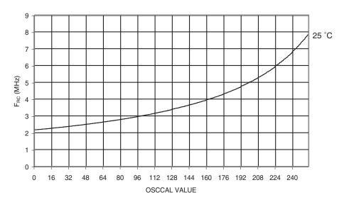
Figure 201. Calibrated 8 MHz RC Oscillator Frequency vs. Temperature
