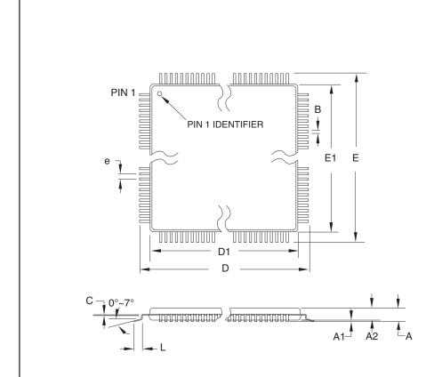
1.This package conforms to JEDEC reference MS-026, Variation AEB.2. Dimensions D1 and E1 do not include mold protrusion. Allowable protrusion is 0.25 mm per side. Dimensions D1 and E1 are maximum
