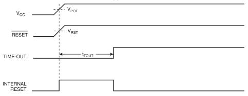
Figure 24. MCU Start-up, RESET Extended Externally
