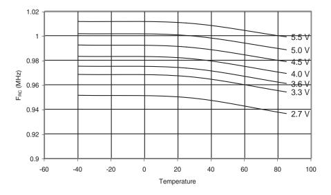
Figure 193. Calibrated 1 MHz RC Oscillator Frequency vs.  $V_{\text{CC}}$
