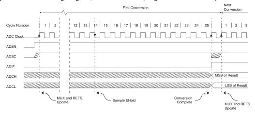
Figure 111. ADC Timing Diagram, Single Conversion
