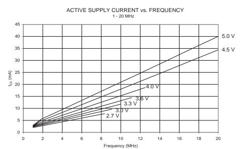
Figure 161. Active Supply Current vs. Frequency (1 - 20 MHz)
