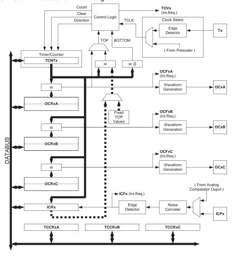
Figure 46. 16-bit Timer/Counter Block Diagram
