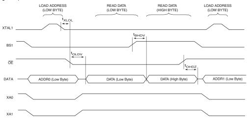
Note: The timing requirements shown in Figure 141 (i.e. t<sub>DVXH</sub>, t<sub>XHXL</sub>, and t<sub>XLDX</sub>) also apply to reading operation.
